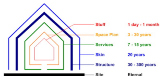
Figuur 5: shearing layers model (Brand, 1994)
